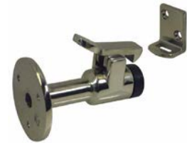
#31.712: Hook door holder spring loaded; Distance 86 mm or 3 3/8" STAINLESS STEEL
